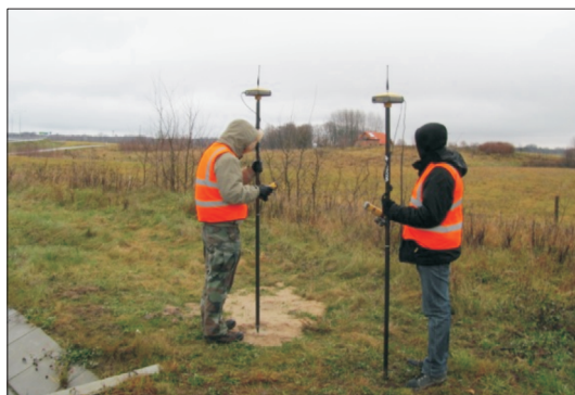
Fig. 3. Survey of points by means of the RTK method
