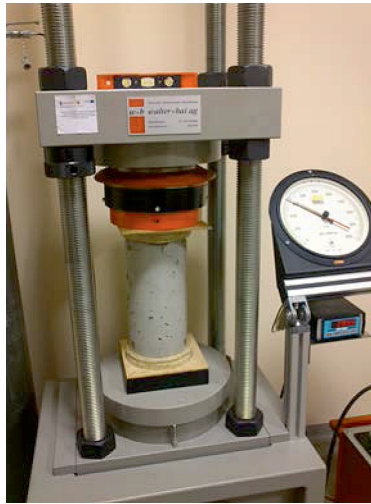
Fig. 1. Concrete creep testing machine Type HKB-1000 kN manufactured by walter+bai ag
