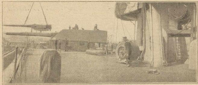
Lifting out one of the twin 14 in. guns on a British warship. The weighty weapon is seen swinging in mid-air as it has been raised by a powerful crane out of its position in the gun-turret.
