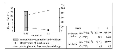
Fig. 4. The average value of the residual ammonium in the effluent, nitrification effectiveness and the contribution of autotrophic nitrifiers in activated sludge depending on VFA/TKN ratio in wastewater (in the table activated sludge and nitrifiers concentrations are shown)
