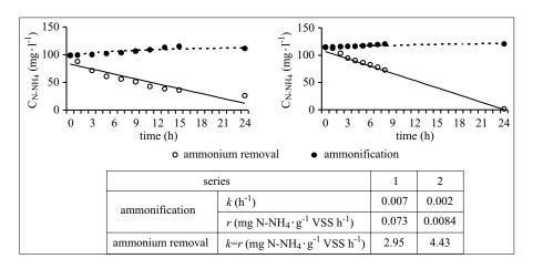
Fig. 2. Variation of ammonium concentration due to ammonification  $(C_{N-NH_4}amon)$  and ammonium removal during the reaction time  $(C_{N-NH_4s})$  a) series 1, b) series 2 (in the table the values of the constant rate (k) and the initial rate (r) are shown)
