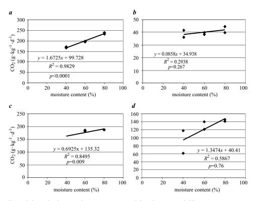
Fig. 2. Relationship between the moisture content of the substratum and  $CO_2$  emission: a – sewage sludge, b – fly ash, c – fly ash + sewage sludge (25% + 75%), d – fly ash + sewage sludge (50% + 50%)
