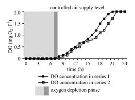
Fig. 1. The duration of oxygen depletion phase and variation of DO concentration in the reactor during the reaction time in series 1 and 2
