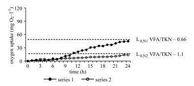
Fig. 3. Oxygen uptake by authotrophs for ammonium oxidation depending on VFA/TKN ratio in wastewater (series 1 and 2)
