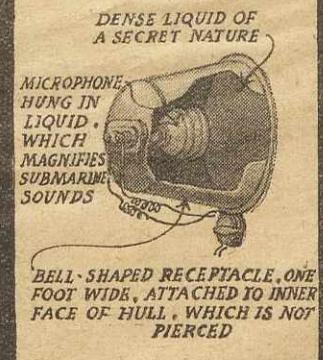
One of the latest suggestions for the detection of submarines at a distance is the application of the microphone, or sound magnifier, for the purpose, so that the sinister craft may be heard though unseen. This very interesting diagram shows the way in which
